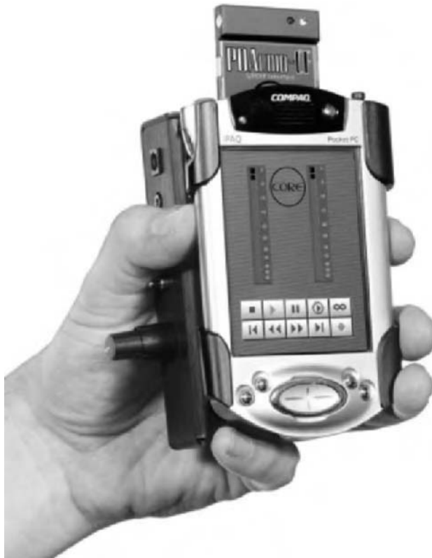
Figure 9.4 PDAudio-CF installed in an HP iPAQ Pocket PC. A Mic2496 preamp/converter is attached to the iPAQ.
